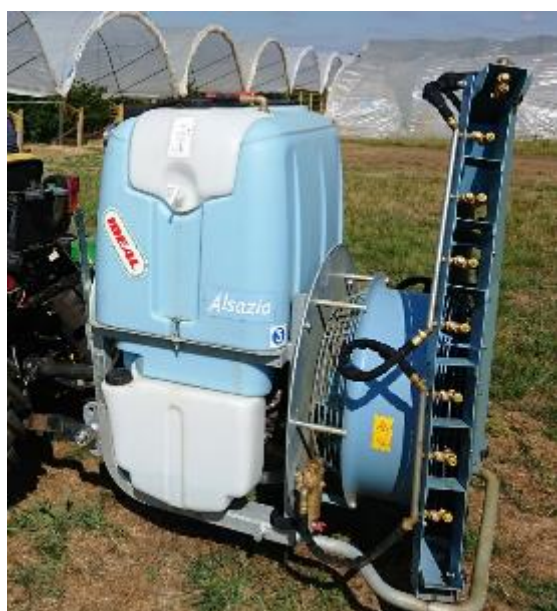
Figure 43: The Ideal Alsazia. A tractor mounted spray machine used during the trials.
