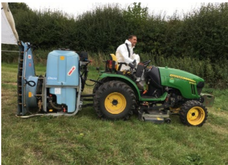
Figure 23. Grower's sprayer used for application of plant protection products.
